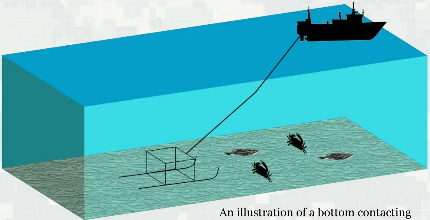
An illustration of a bottom contacting benthic sled towed along the seafloor. The sled is usually equipped with an image sensor.
