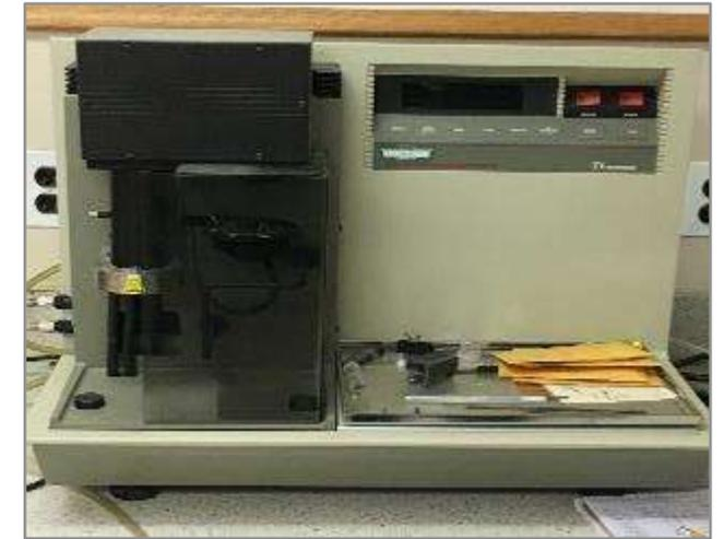
Thermal Gravimetric Analyzer
