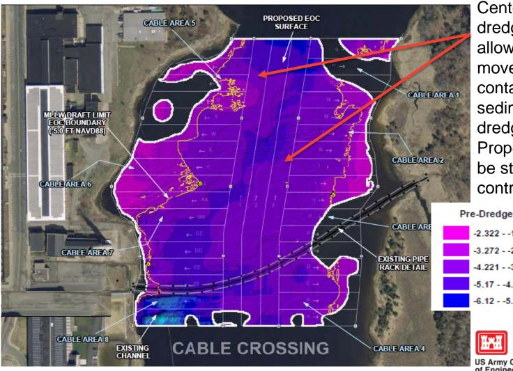
Center lanes will be dredged first to allow vessels to move with moving contaminated sediment within dredge area. Propeller was will be strictly controlled.
