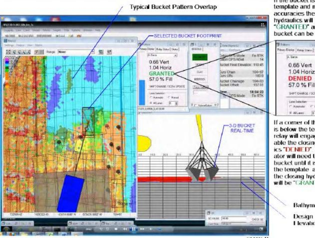
If the bucket is within the template and meets the accuracies the closing hydraulics will be "GRANTED" and a bucket can be taken
