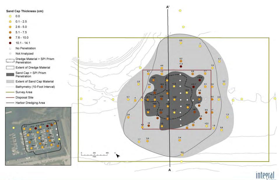
Mapping Disposed Dredged Material and a Sand Cap for the Douglas Harbor Dredging Project Using SPI and Semiautomated Image Processing System
