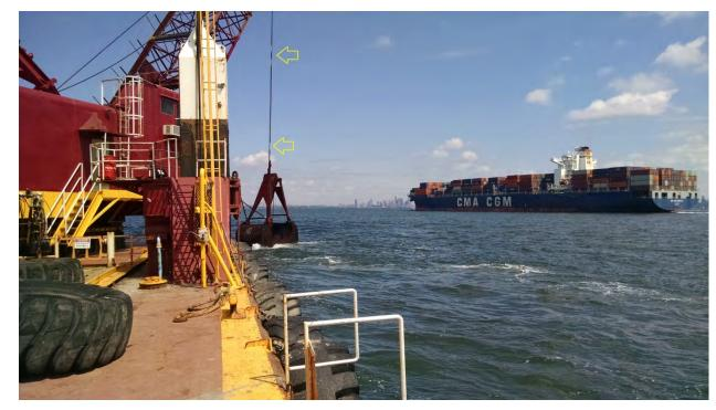
Figure 8. Dredging Operation in Progress (yellow arrows indicate cable markings for depth control and dredge bucket open/close check)
