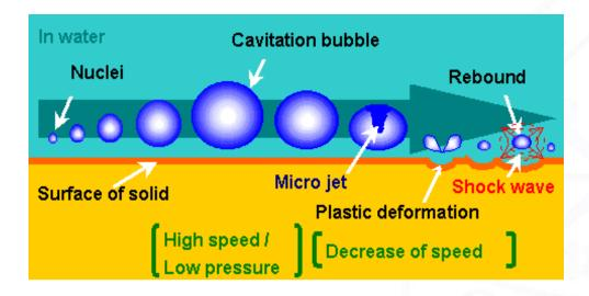
The jets will create a stream of cavitation bubbles which will further reduce the particle size.
