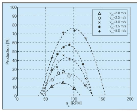
Production versus RPM of cutter head for different mixing suction velocities
