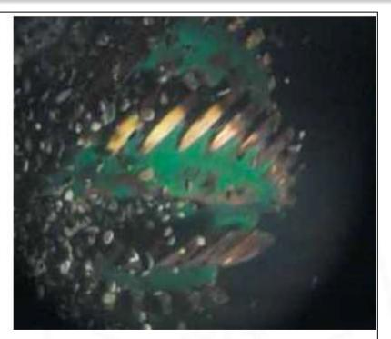
Cutter Head 90 RPM Note: Particles being thrown out near the cutter ring and before suction intake
