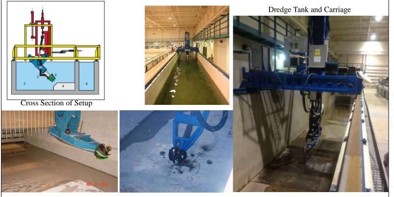
Rotary Cutter Head Setup in Tank
