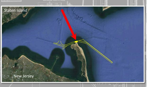
Scope of Work **O&M** Dredging Quantity: 250,000 CY Material Type: Sand **Placement Areas:** Ocean Mechanical **Equipment: Environmental** 15 November – 15 Windows: September Advertisement June 2017 Date: Bid Opening Date: July 2017 Start Date: September 2017 (NTP) Issues: None
