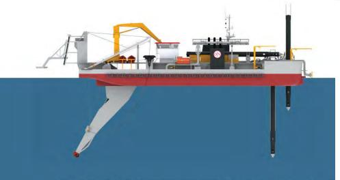
Dynamically controlled flexible spudcarrier: active control of longitudinal movement and force, of the roll angle and moment, of the pitch angle and moment.
