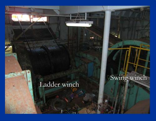
Equipment: Ladder lifting winch Ladder Swing winch Spud winch Stern winch Bearing : Electric motor (gear) Reducer Pinion Winch drum Vibration : 15points : 33points AE
