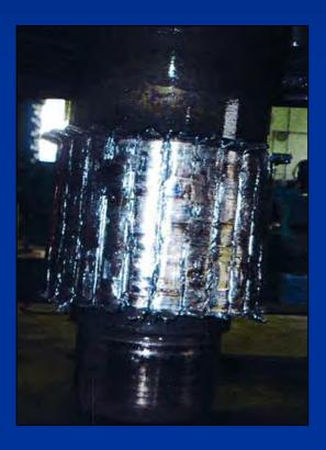
Type: Cutter Suction DredgerEquipment: Ladder Lifting WinchDamaged parts: The Sun gear of the<br/>planetary reduction gearsMaterial: SCM21<br/>(Chromium molybdenum steel)
