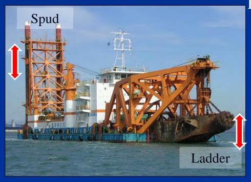
Equipment: Ladder lifting winch Ladder Swing winch Spud winch Stern winch Bearing : Electric motor (gear) Reducer Pinion Winch drum Vibration : 15points : 33points AE
