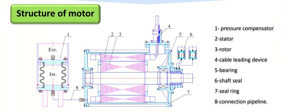
◆The inner chamber of motor is connected to a pressure compensator mounted outside of motor with a pipeline providing two-way flow and sealing.
