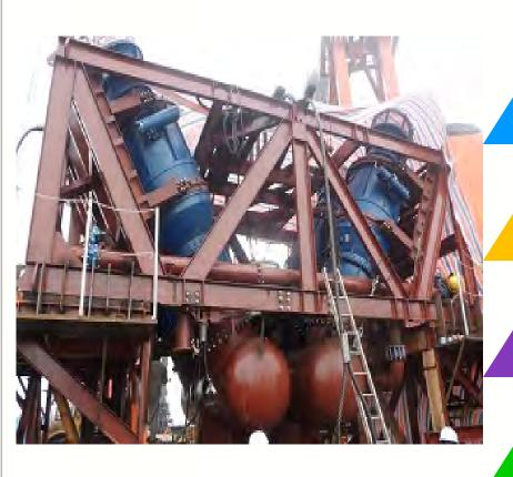
The equipment opens ditches using water flow from the pumps in order to lay petroleum pipelines in the seabed.
