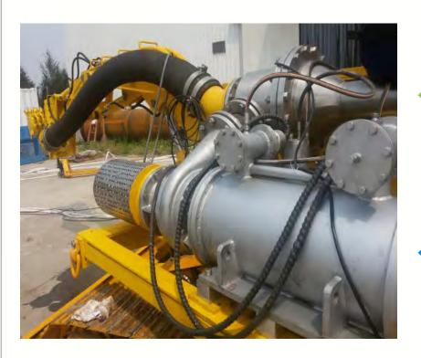
The under water electric motor drives an hydraulic pump supplying power to hydraulic machine hands.
