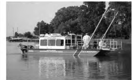
EPA's research vessel Mudpuppy can enter shallow inlets on the Great Lakes to test for contaminated sediment.
