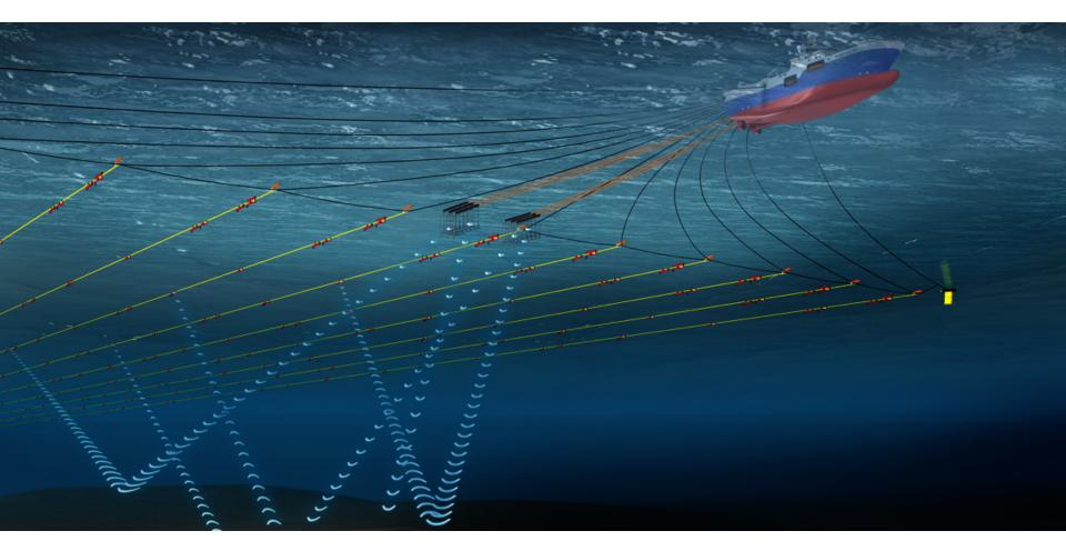
Seabed geophysics may use active or passive methods. Acoustic signal reflection, refraction, electro-magnetic resistivity and passive magnetometers make up the most common methods.
