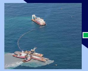
Cutterhead Dredge Excavation and Filling Scow Barge via Spider Barge
