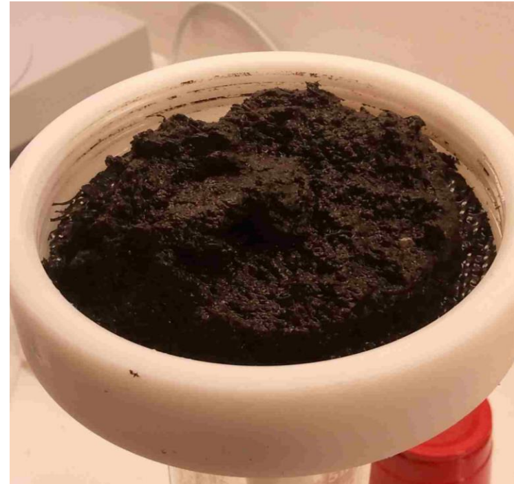
Captured filtrate and solids after chemical conditioning and poured through GT500
