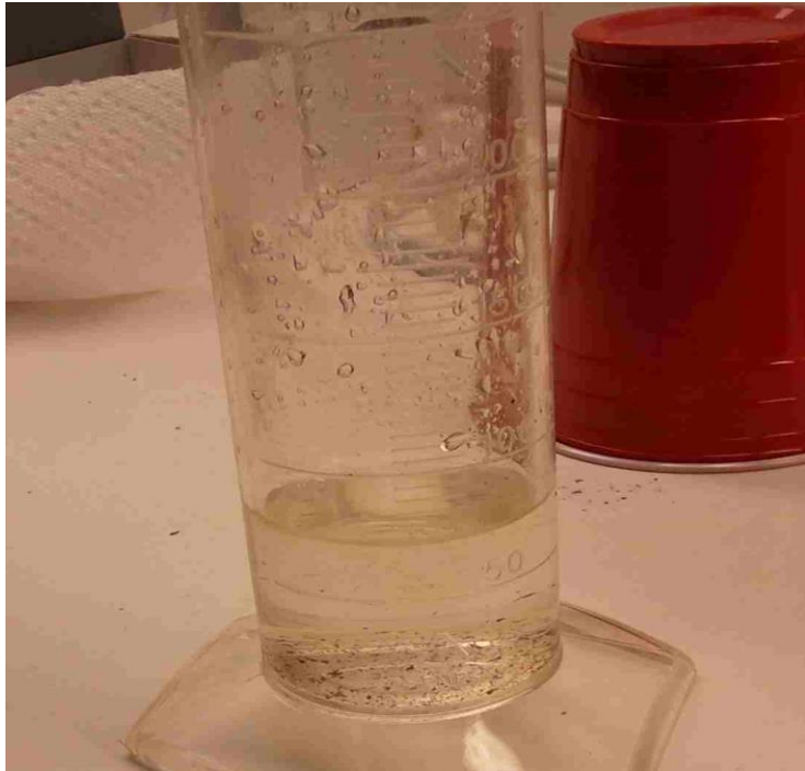
Captured filtrate and solids after chemical conditioning and poured through GT500
