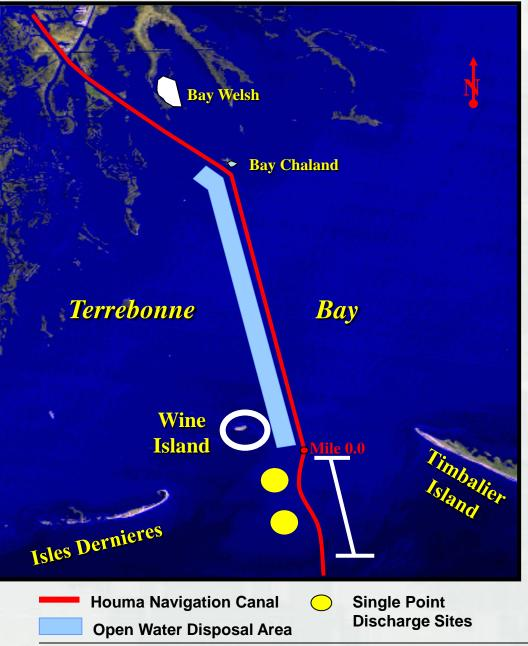
HOUMA NAVIGATION CANAL New Orleans Harbor #3-2013 **Terrebonne Bay & Cat Island Pass** Type of Equipment: Cutterhead Schedule: Aug 2013 **Depth:** 17 ft – 22 ft **Width:** 150 ft – 300 ft Quantity: 1.5 M cubic yards Placement Area: Open Water /SPD/Barrier Island Restoration **Distance to Placement Area:**
