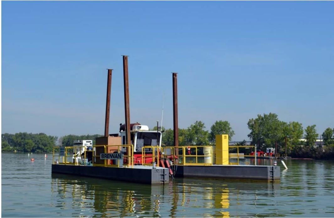
**Photo 4. Eight-inch swinging-ladder hydraulic dredge removing non-TSCA sediment.**
