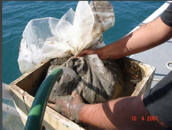
Nylon sieve (500 \mu m mesh size)
