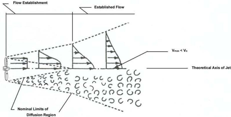
**Figure 1. Geometry of initial velocity zone and momentum jet formed by propulsion system.**
