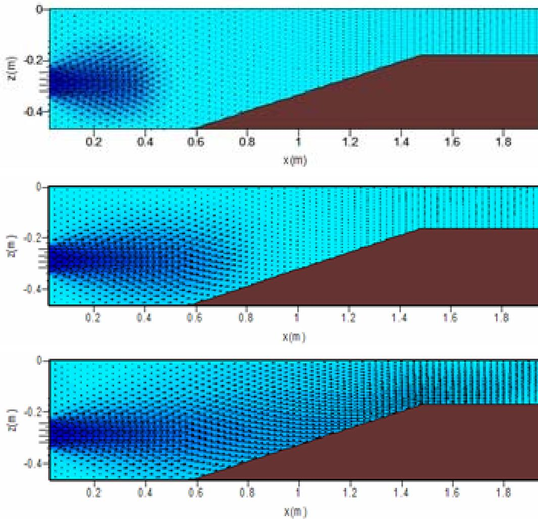
Figure 5. Vertical cross-sections of velocity at time a) 0.95 sec, b) 2.35 sec and c) 9.50 sec
