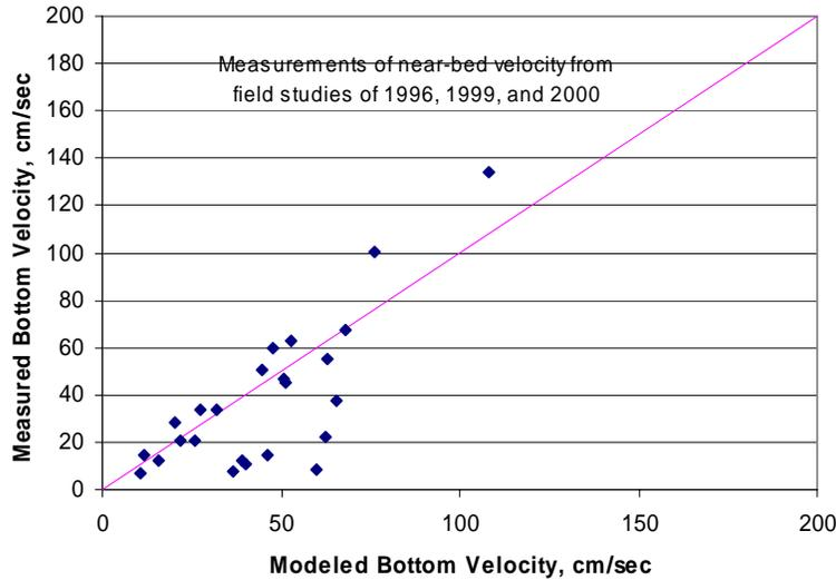
Figure 2. Comparison of VH-PS model predicted and measured propeller wash bottom velocities.
