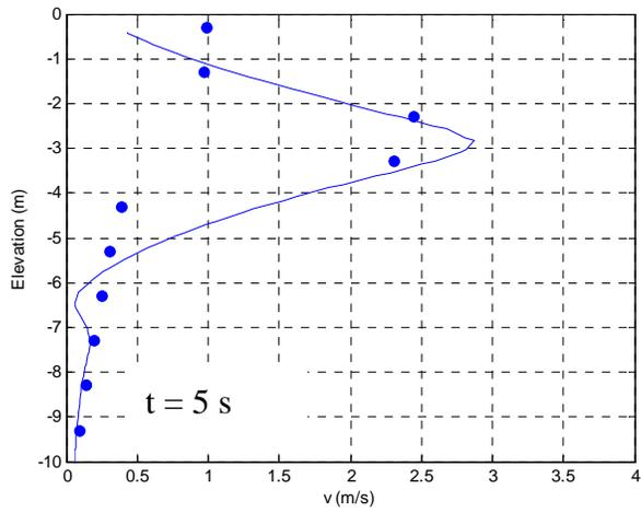
**Figure 10. Comparisons of measured and predicted velocities in the vertical cross-section at the propeller axis for test 2. Solid lines are computations, dots are field data.**
