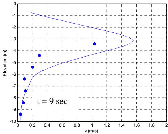
**Figure 9. Comparisons of measured and predicted velocities in the vertical cross-section at the propeller axis for test 1. Solid lines are computations, dots are field data.**
