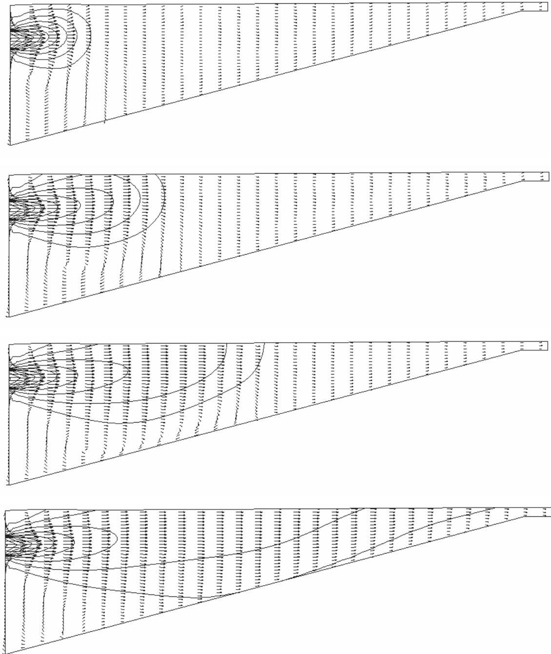
**Figure 8. Vertical cross-sections of velocity at the propeller axis for test 2 and time a) 5 sec, b) 15 sec, c) 30 sec and d) 80 sec. Maximum jet velocity is 5.0 m/s with contours at 0.5 m/s intervals.**
