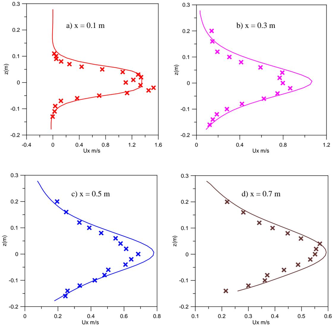
**Figure 6. Vertical distributions of mean measured and predicted velocities along the jet axis at varying distance from the propeller. Solid lines are computations; crosses are lab data Schokking (2002).**
