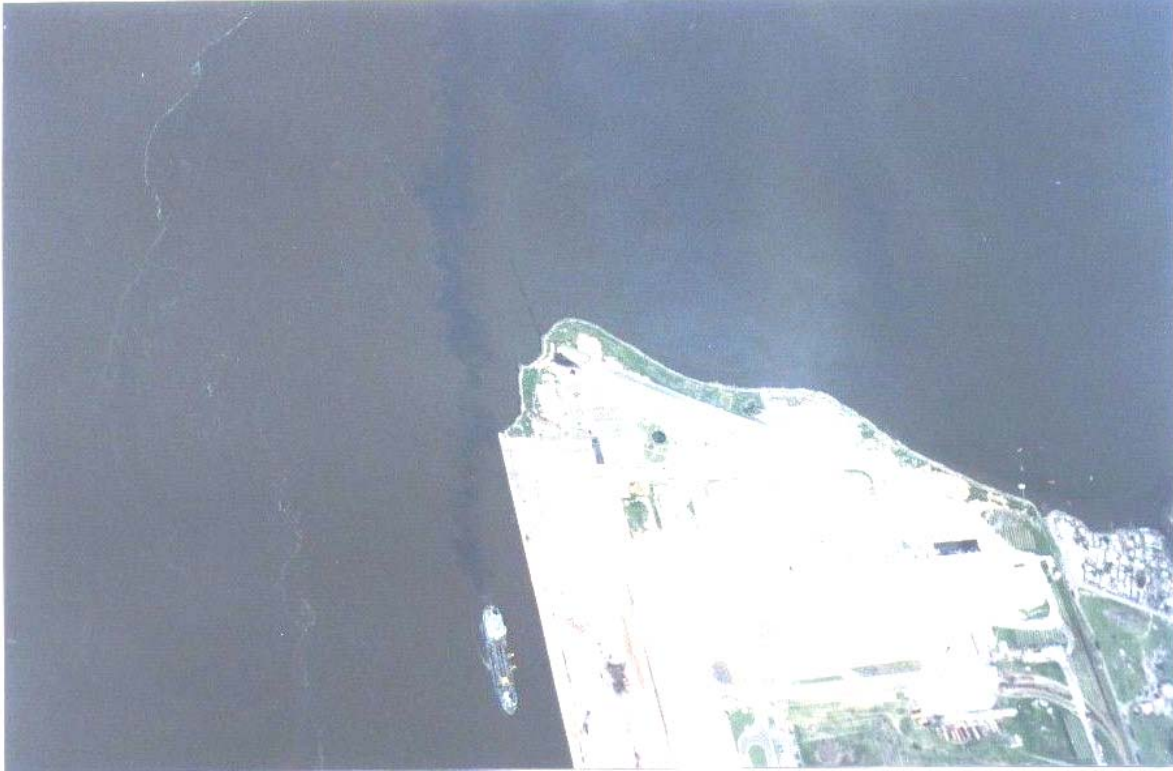
Figure 4. Picture of the dredge working on the Porto Novo in 2000 showing the turbidity plume behind the dredge (Asmus and Zamboni 2001).
