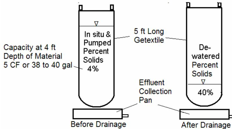
**Figure 5. Schematic drawing of the hanging bag before and after drainage**
