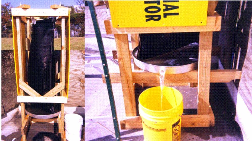
**Figure 7. Includes the bag hanging in a wooden frame and clear effluent collecting in the pan and bucket**
