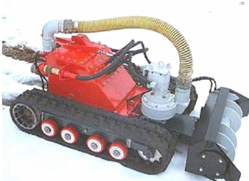
**Figure 8. Typical submersible hydraulic track dredge and suction cutterhead (ref. Liquid Waste Technology)**
