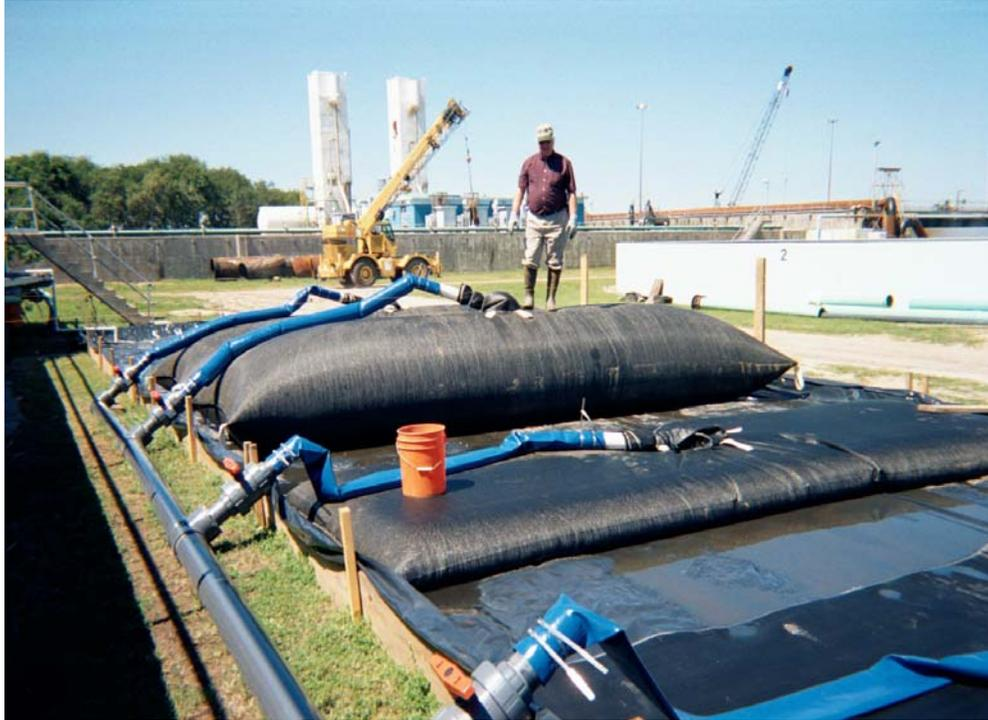
**Figure 11. Filling 15 ft circumference diameter tubes to evaluate dewatering capabilities**
