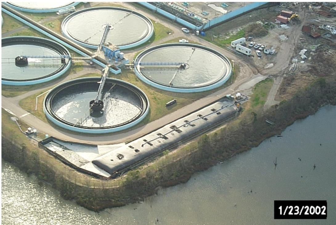
**Figure 14. Aerial view of clarifiers and 27 m (90 ft) circumference 82 m (270 ft) long geotextile tube filled to a height of 2 m (7 ft)**
