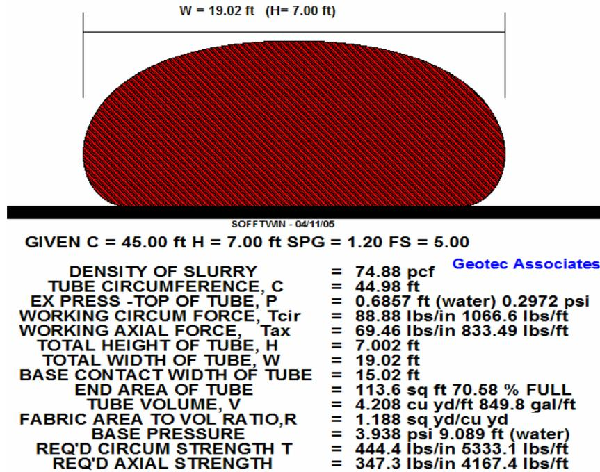
**Figure 6. Cross section of a 13.5 m (45 ft) circumference geotextile tube used to dewater biosolid sediments**
