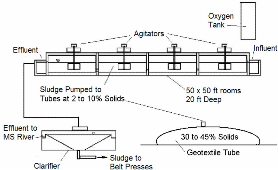
**Figure 4. Schematic view of four out of eight aeration chambers, oxygen tank, clarifier and geotextile tube**
