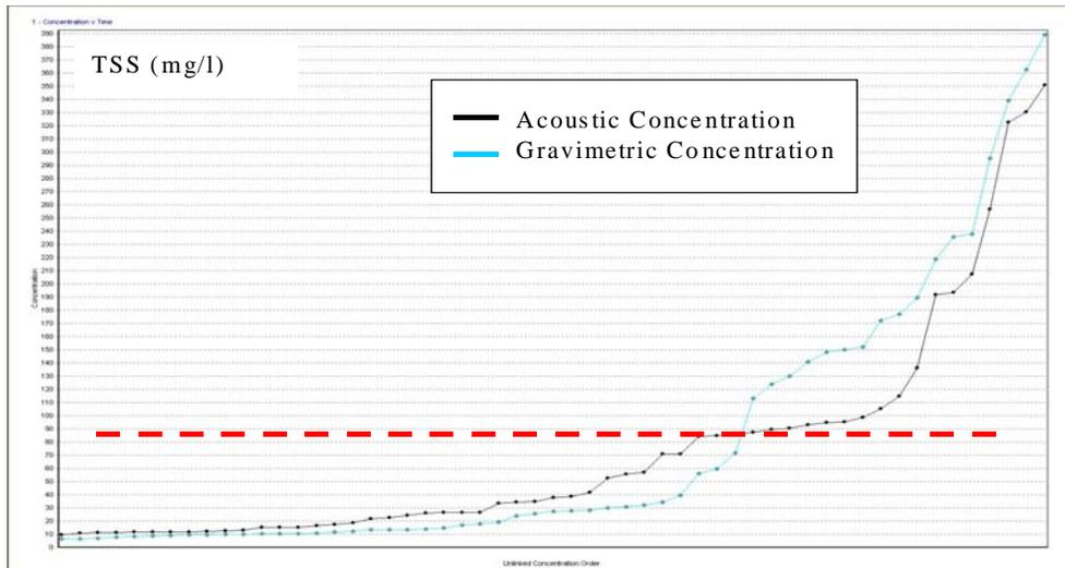
Figure 2. Comparison of acoustic and gravimetric measurements of suspended sediment concentration in rank order.
