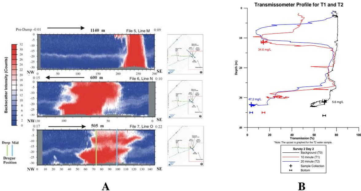
**Figure 6. Profile plots of ADCP data collected along Lines M, N, and O (Plume 2) displaying residual acoustic backscatter intensity within the water column to illustrate plume morphology prior to disposal and 22 minutes after the dredged material disposal event at Point A (A). Profile plot of percent light transmission and sensor depth acquired during CTD sample intervals T1 and T2 for Plume 2 (B).**
