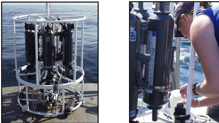
**Figure 3. Images of the Seabird SBE32 Carousel unit employed as part of the plume monitoring surveys performed at RISDS.**
