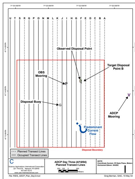
Figure 2. Basemap displaying a subset of the predetermined ADCP survey lanes established over RISDS.
