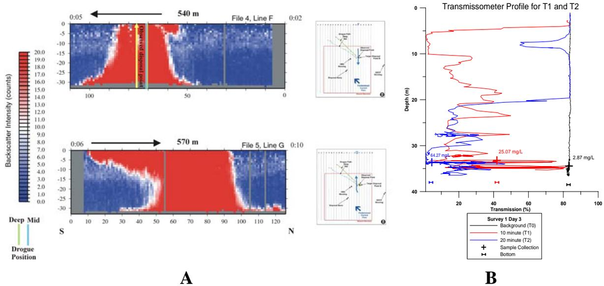
**Figure 4. Profile plots of ADCP data collected along Lines F and G (Plume 3) displaying residual acoustic backscatter intensity within the water column to illustrate plume morphology 2 to 10 minutes after the dredged material disposal event at Point B (A). Profile plot of percent light transmission versus sensor depth acquired during CTD sample intervals T1 and T2 during Plume 3 (B).**
