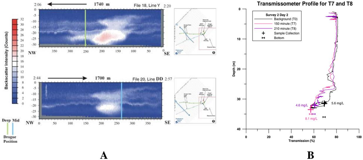
**Figure 7. Profile plots of ADCP data collected along Lines Y and DD (Plume 2) displaying residual acoustic backscatter intensity within the water column to illustrate plume morphology 126 to 177 minutes after the dredged material disposal event at Point B (A). Profile plot of percent light transmission and sensor depth acquired during CTD sample intervals T7 and T8 for Plume 2 (B).**
