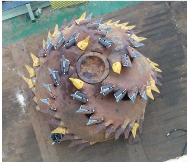
Figure 2. VOSTA D65 test cutterhead equipped partly with T6.30 tube adapters (prototypes)
