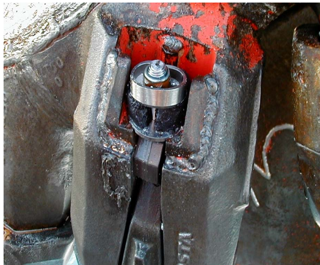
Figure 11. Showing damaged locking ring and rubber
