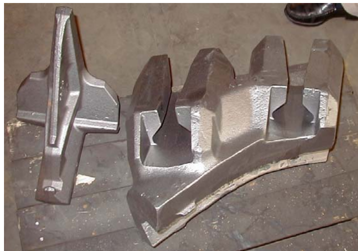
Figure 13. The twin adapter for the teeth on POS 1 and 3
