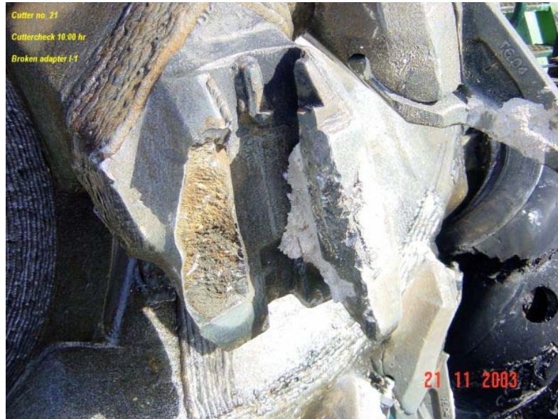
Figure 12. Showing the broken side support of the adapter
