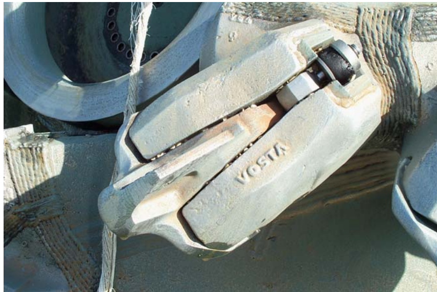
Figure 5. Top view on adapter showing the slots that create the flushing effect. The few small particles in the open slots have no influence.
