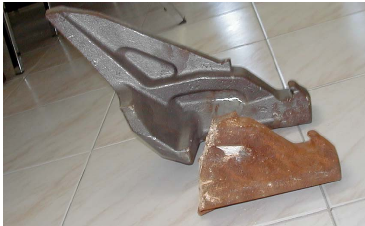
Figure 9. Tooth broken in the coupling part
