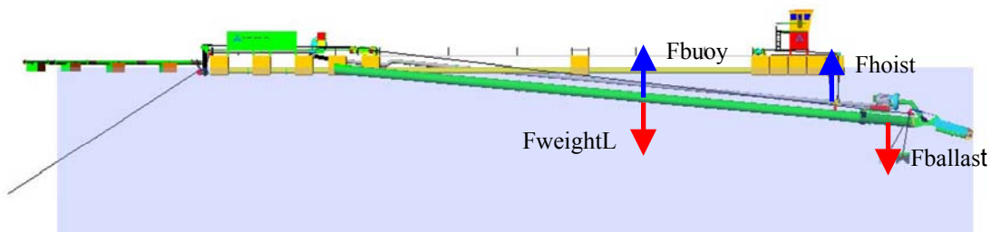
Figure 3: Simple force balance during ladder hoisting lowering
