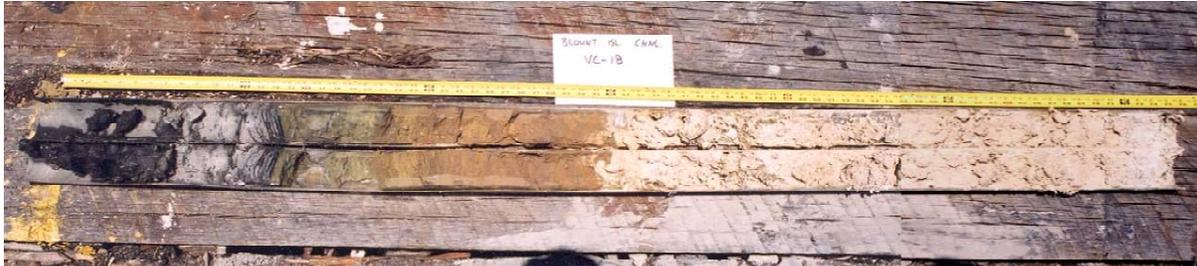
Figure 8 - Vibrocore photo log
