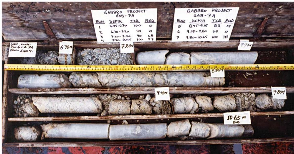
Figure 9 - Rock core photo log
