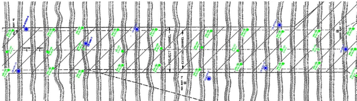
Figure 10 - Jet probes (in green) supplementing borings (blue)
