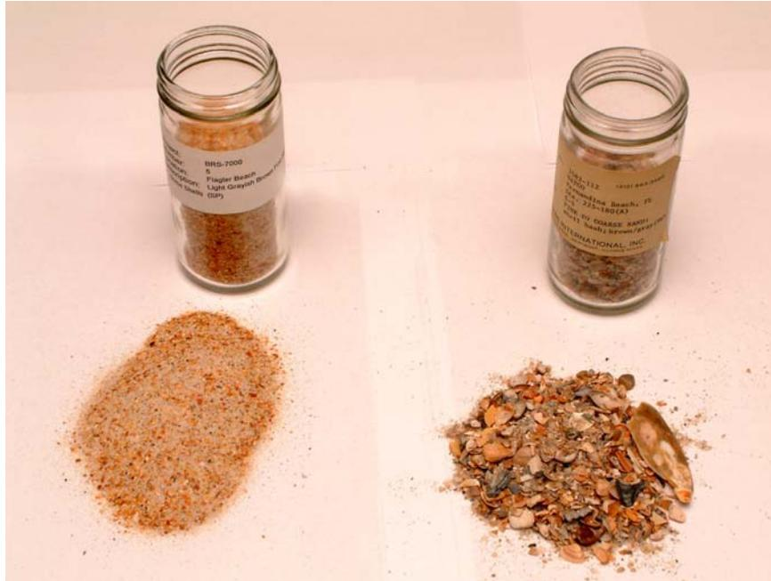
Figure 13 - Sand samples described as Sand with "some shell" (left) and with "shell hash" (right)
