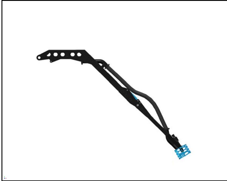
Figure 1. Ladder extended for dredging in the forward direction
