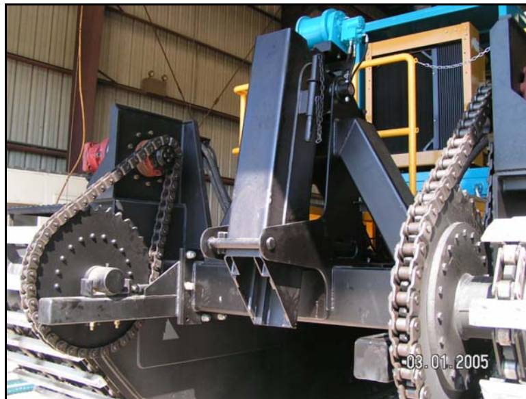
Figure 4. Kicker spud assembly tilted in the forward position
