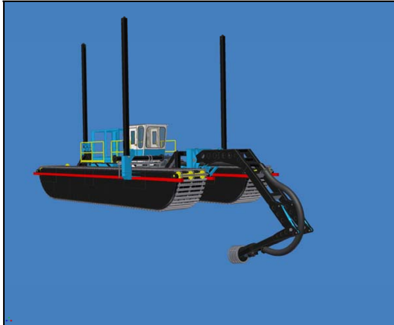
Figure 3. The Amphibian's three-spud system
