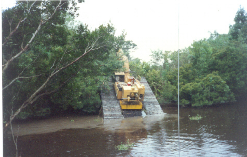
Figure 5. Track mounted hydraulic excavator shown climbing from a freshwater lake
