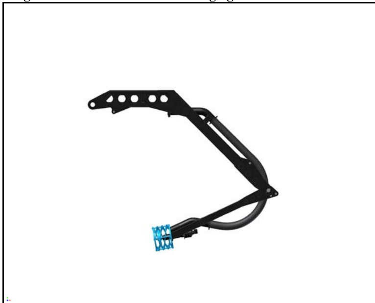
Figure 2. Ladder manipulated for dredging in the reverse direction
