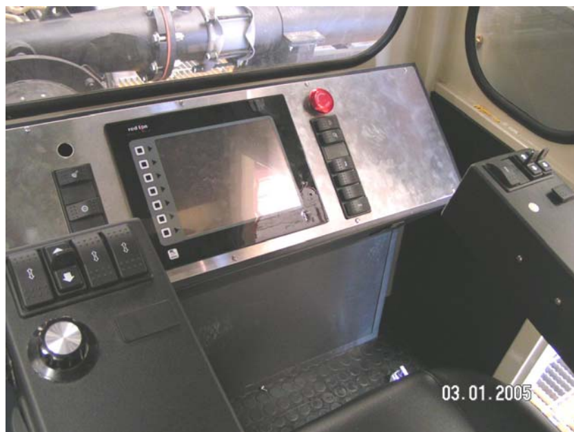
Figure 9. Operator control console with ergonomically designed operator chair and touch screen.
