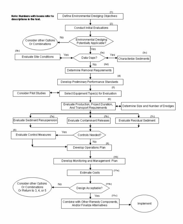
Figure 1. Flowchart illustrating environmental dredging design sequence.
