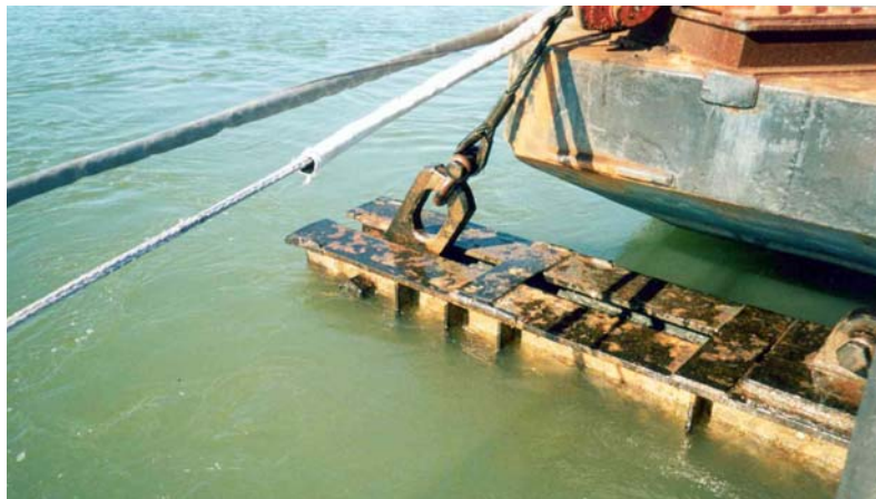
Figure 3. One end of the knockdown bar suspended from the barge at the water surface.
