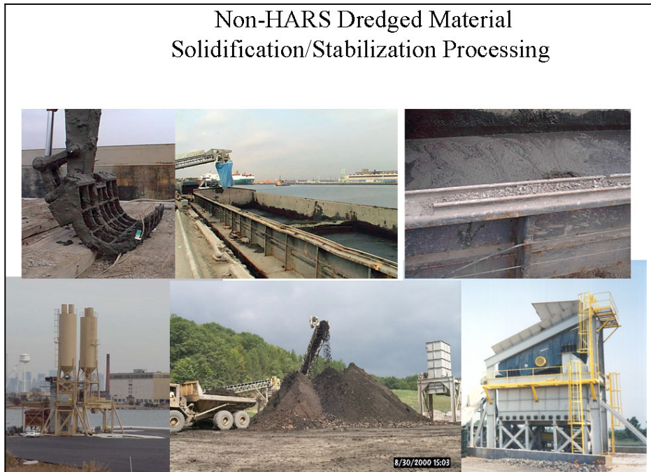
Figure 5. Top. In-barge treatment and stabilization of dredged material with Portland cement. Bottom. Using a pug mill to treat and stabilize dredged material with Portland cement.
