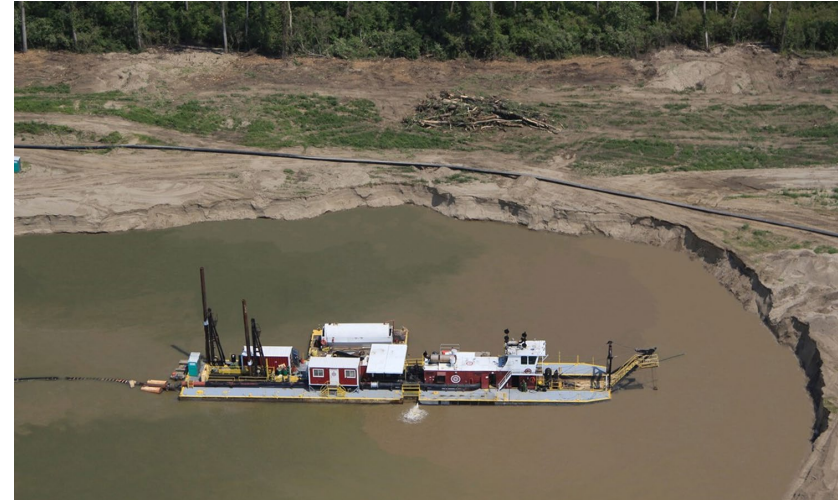
20' Portable Diesel Dredge Sandpiper digging pond Photo by GLDD
