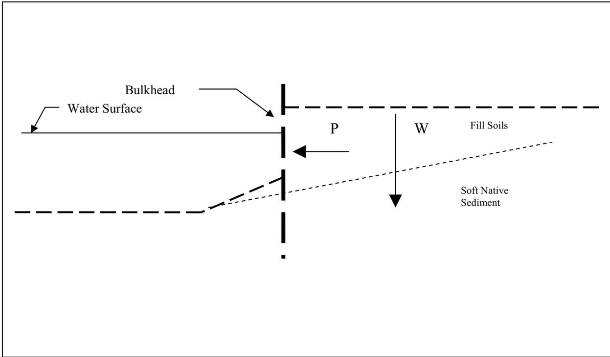
**Figure 1. Typical industrial waterfront cross-section.**
