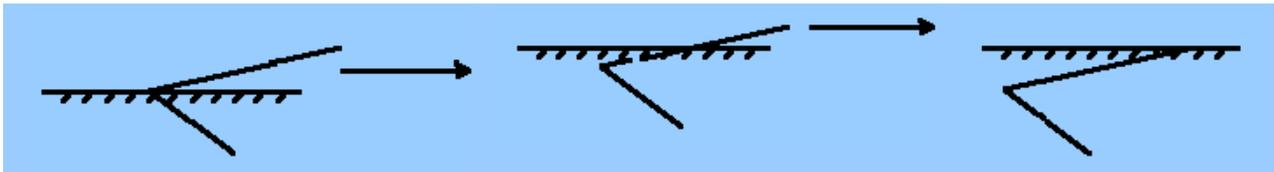
**Figure 9. The shank penetrating the soil in phase 3.**
