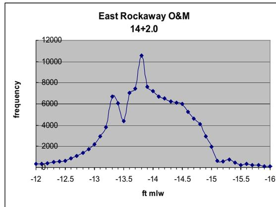
**Figure 11 – Distribution Curve of after-dredge depths for East Rockaway 2005 (1 ft. = 30.5 cm)**
