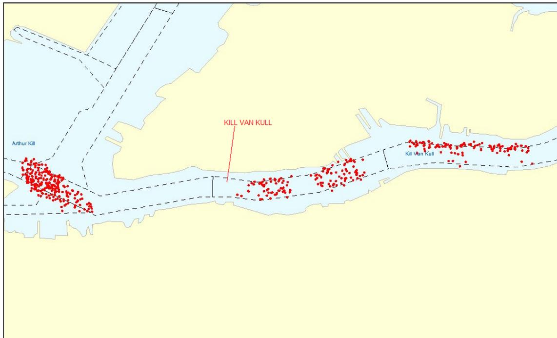
**Figure 3. Online view of loading points illustrating scow positions during loading phases. The cumulative plot demonstrates coverage of dredging and exhibits progress over the Kill Van Kull waterway dredging area in New York.**
