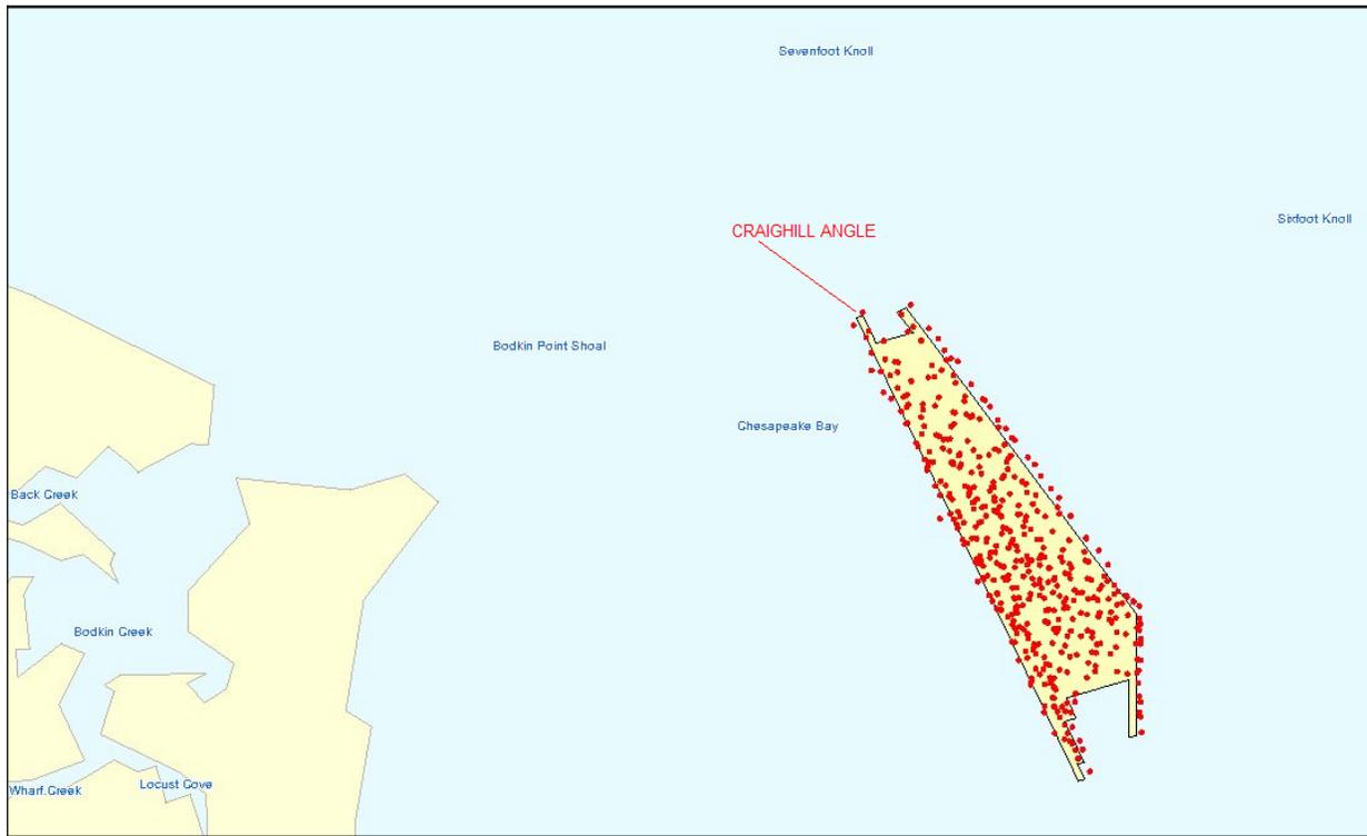
**Figure 2. Online view of loading points illustrating scow positions during loading phases. The cumulative plot demonstrates coverage of dredging and exhibits progress over the Craighill Angle dredging area in Maryland.**
