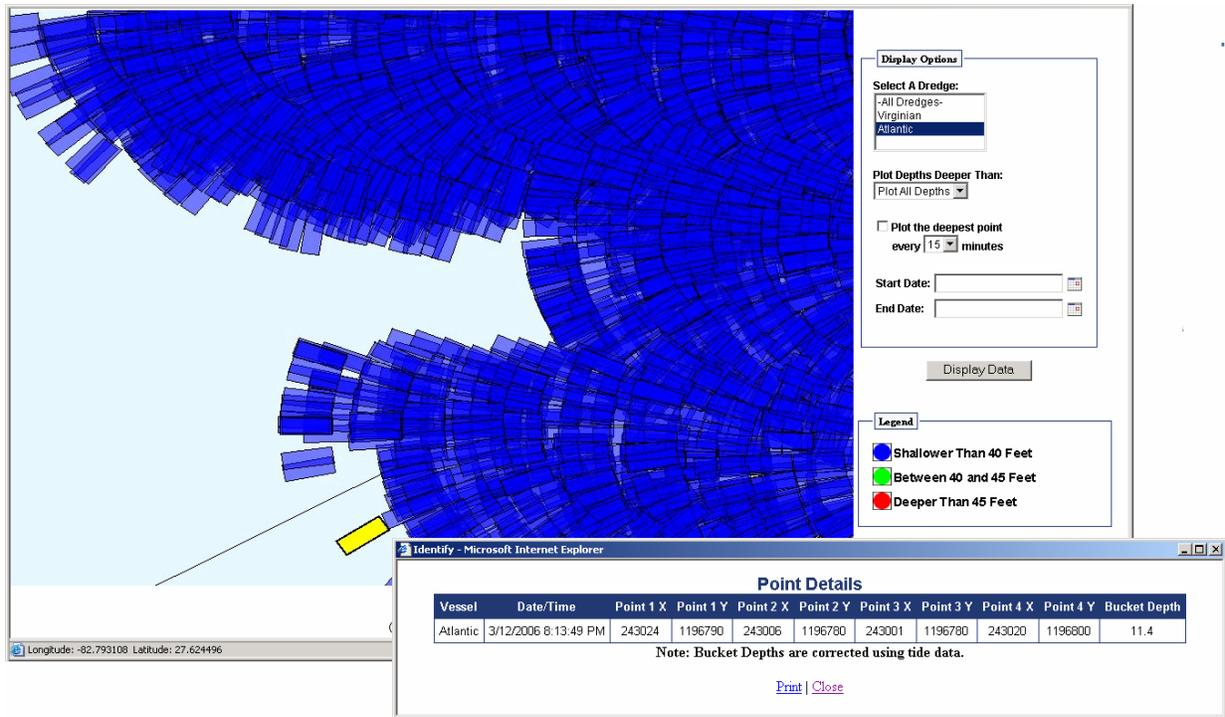
**Figure 6. Online view of imported ClamVision™ log data illustrating bucket coverage. Point details are associated with the highlighted bucket sample.**
