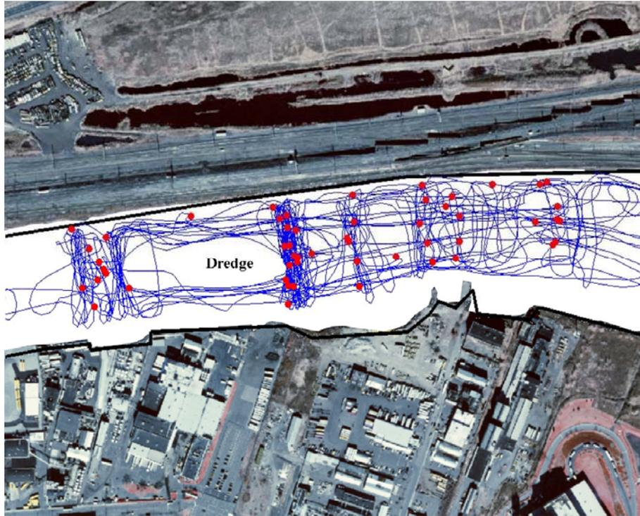
**Figure 11. R/V Caleta December 5, 2005 ship tracks (blue lines) and CTD casts (red dots).**
