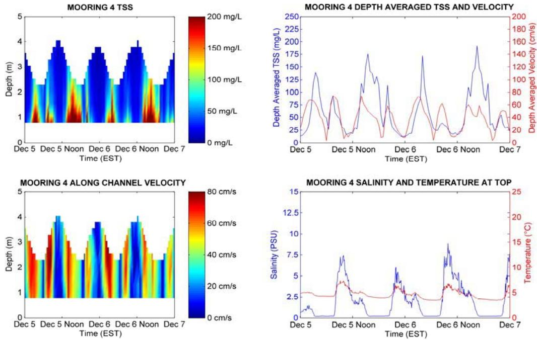
Figure 9. During dredging (first two days) monitoring measurements at mooring 4.
