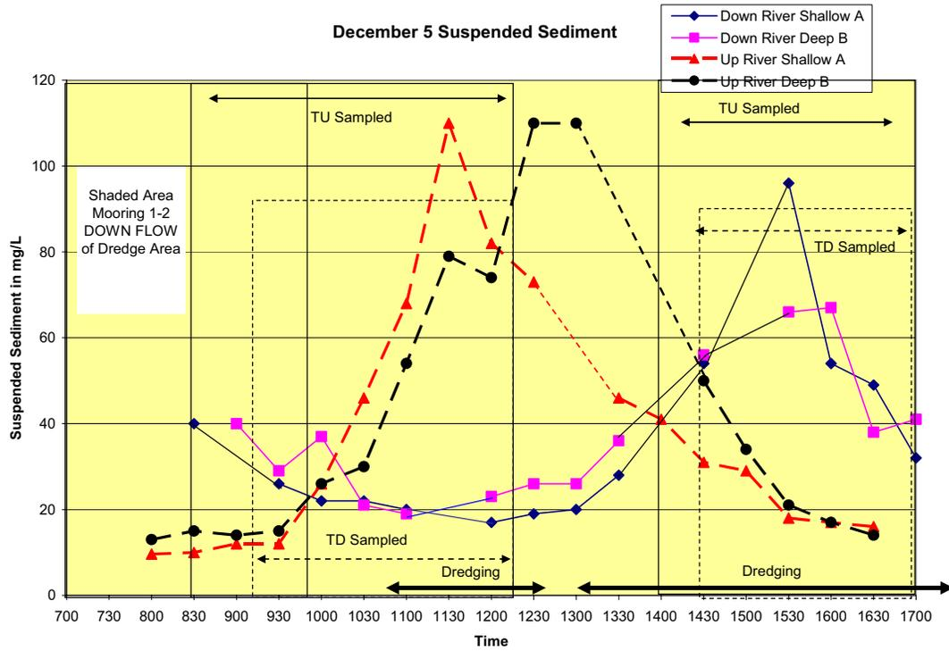
Figure 17. Measurements made by TOPS Boats on December 5, 2005.
