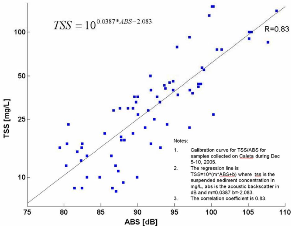
**Figure 14. TSS calibration plot for the R/V Caleta ADCP measurements.**
