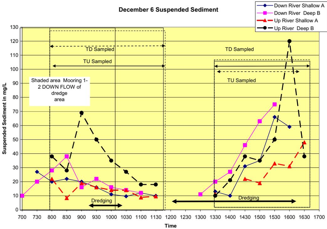
Figure 18. Measurements made by TOPS Boats on December 6, 2005.
