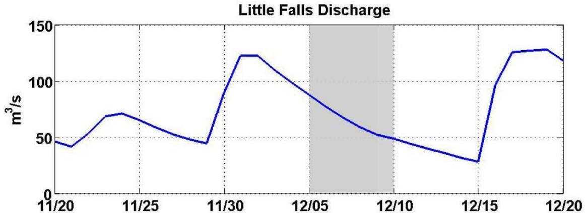
Figure 6. Freshwater discharge measured at the USGS gauge in Little Falls, New Jersey.
