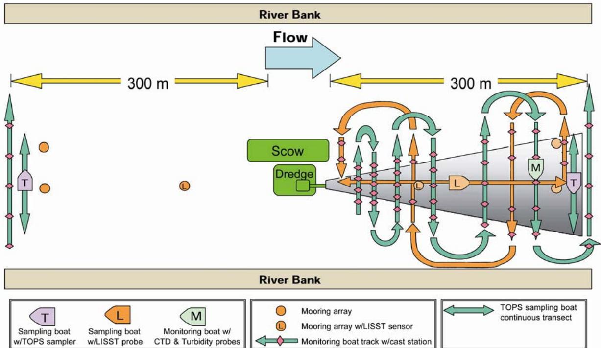
**Figure 5. Monitoring mooring arrangement with monitoring boat track.**
