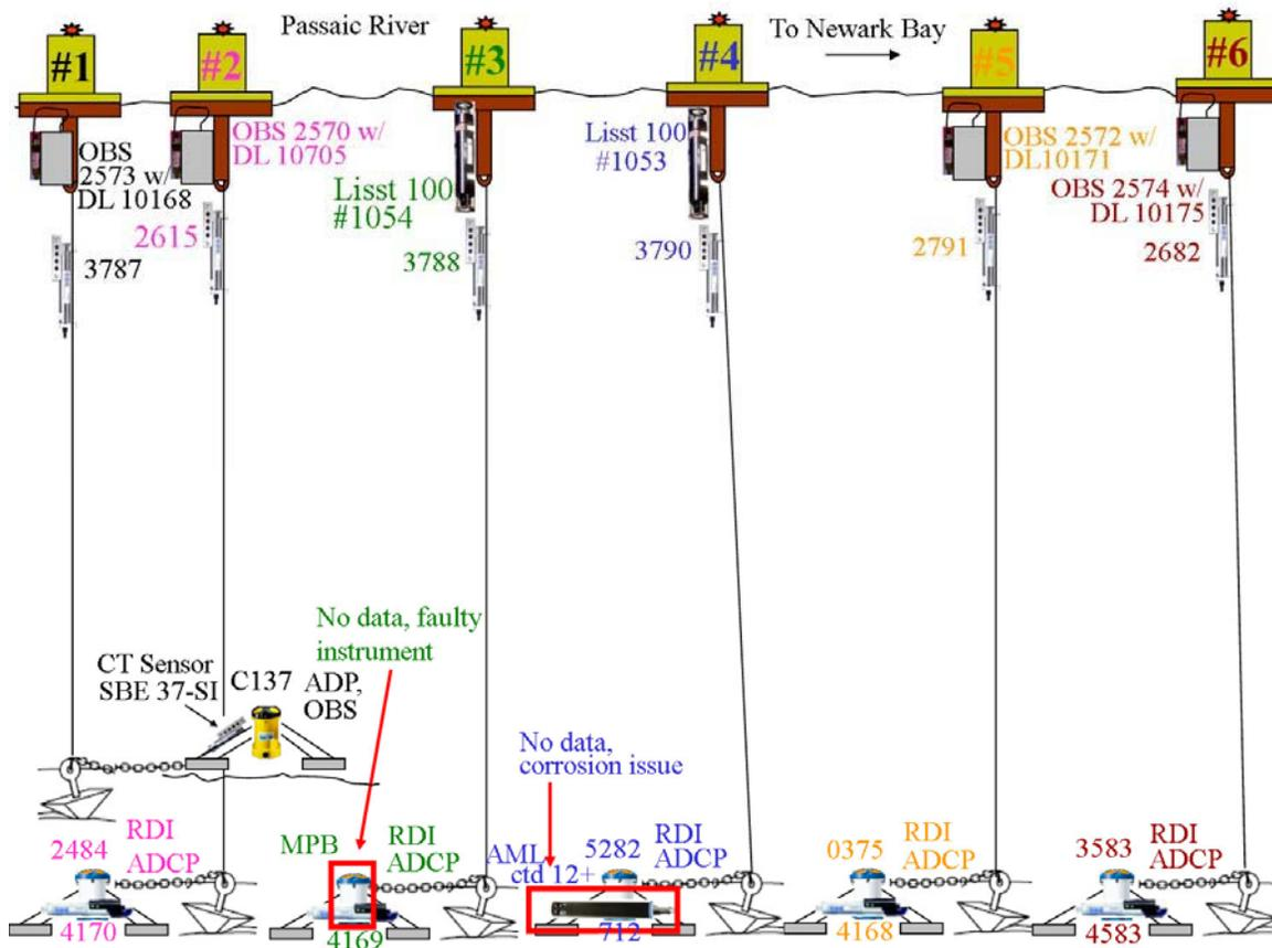
Figure 4. Six Moorings with instruments, floats, anchors, and tripod frames.
