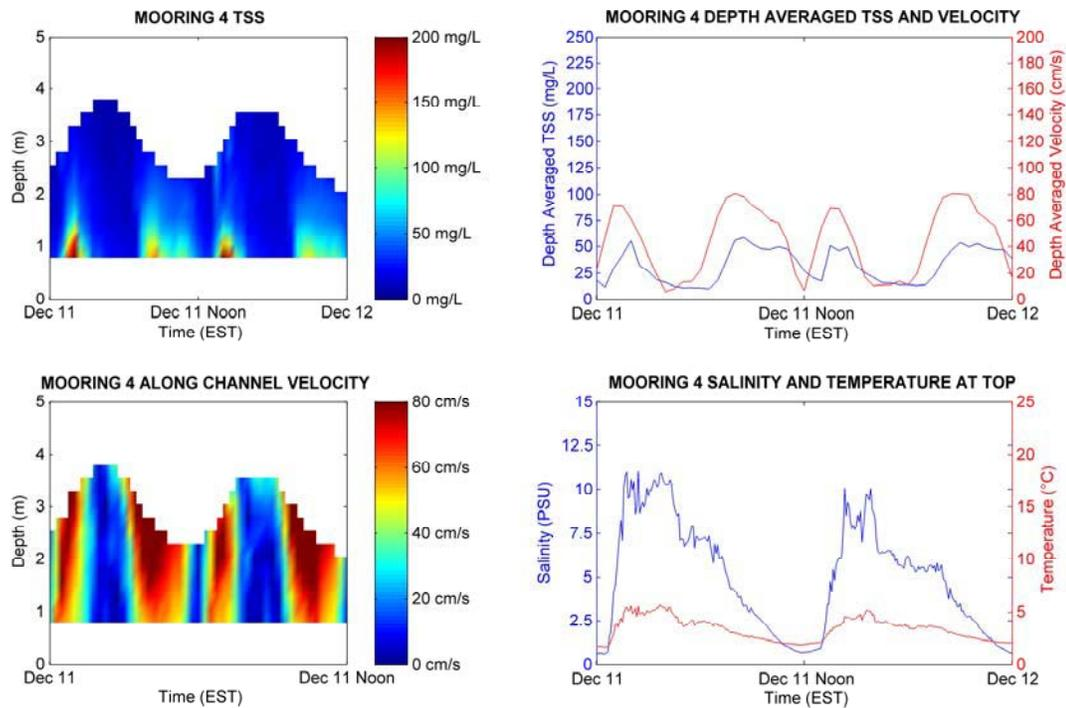
Figure 10. Post dredging monitoring measurements at mooring 4.
