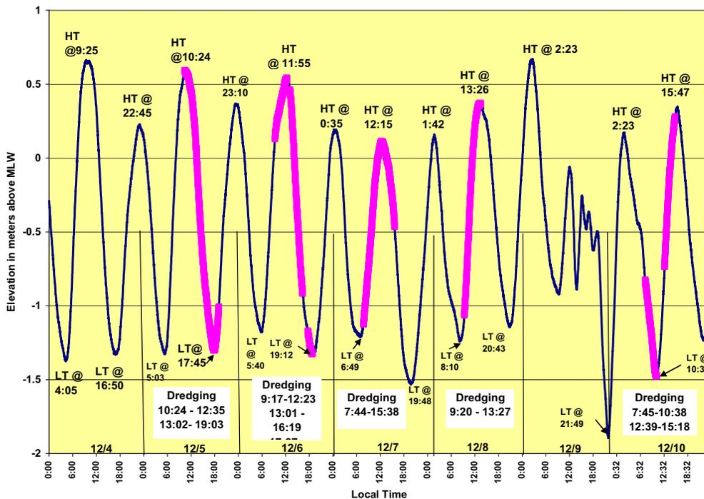
Figure 7. Water surface elevation measured at mooring 2.
