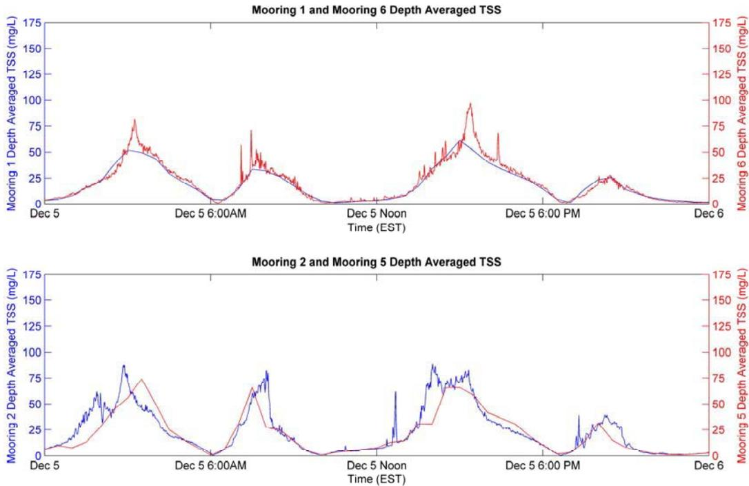
Figure 15. Comparison of depth averaged TSS at moorings 1 & 6 (top panel) and moorings 2 & 5 (bottom panel).
