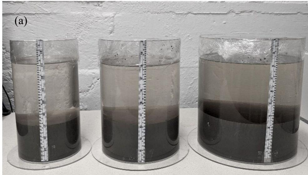
(a) The self-weight consolidation/settling column tests using acrylic plexiglass cylinders with diameters 10", 8", and 6" (Right to left).
