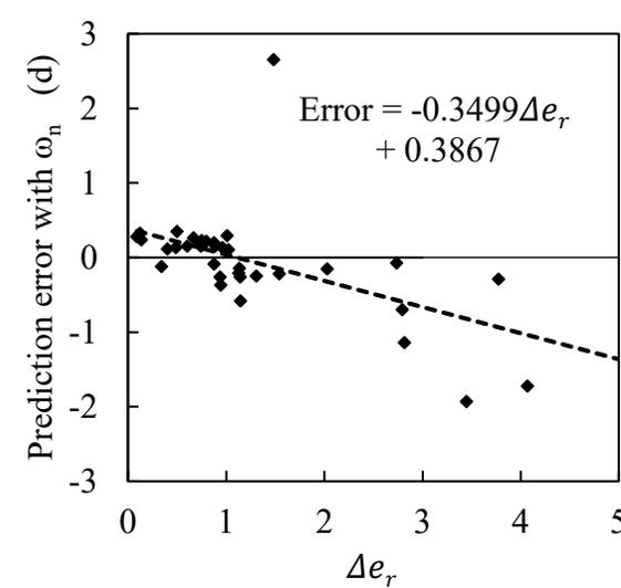
(a) compression index with liquid limit; (b) error of prediction on liquid limit basis vs  $\Delta e_r$ ; (c) compression index with natural water content; (d) error of prediction on natural water content basis vs  $\Delta e_r$ .
