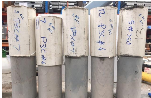
Samples were processed on barge and shipped to laboratory for UCS testing within 2 to 7 days after mixing
