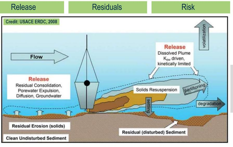
Figure 1. Schematic of contaminant release sources and mechanisms.
