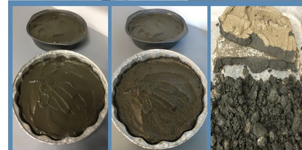
7.5% Portland cement Immediately Post-mixing
