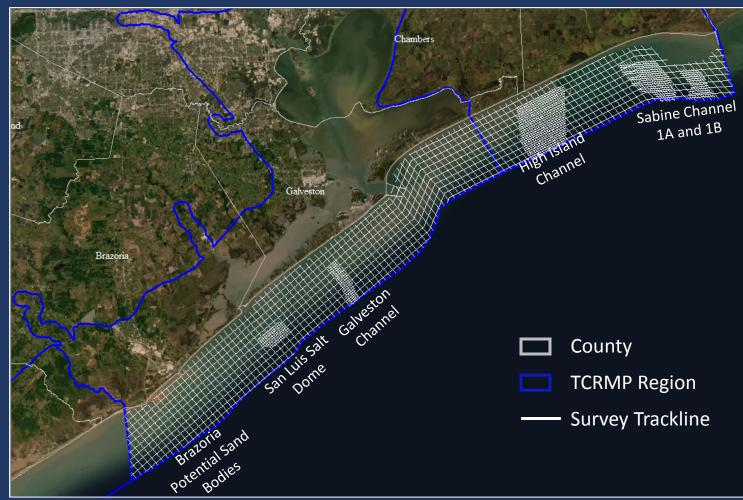
High-resolution geophysical survey tracklines and zoom-in lines
