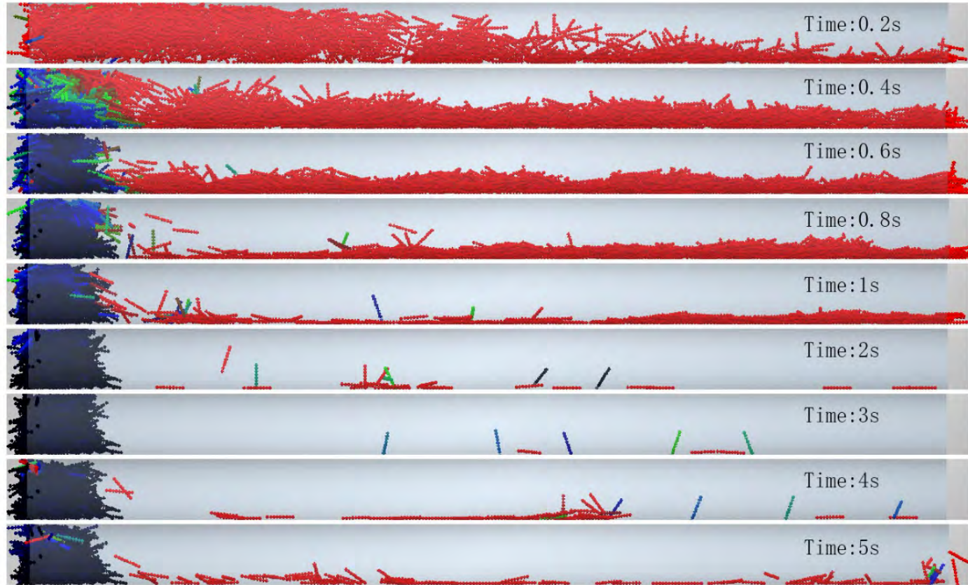
The blockage of long coarse-particles at line speed ( 8m/s ): flocculating + interlocking
