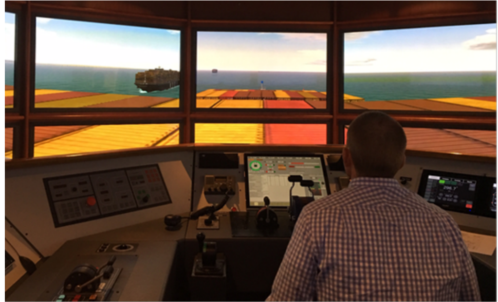
Figure: Full-mission ship simulator at MITAGS
