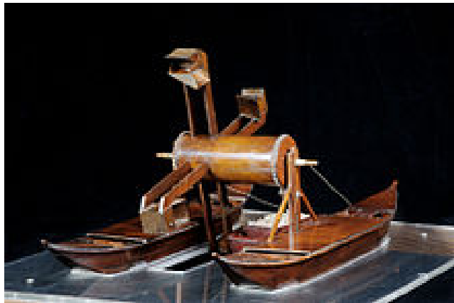
Reconstruction of the mud-drag by Leonardo da Vinci
