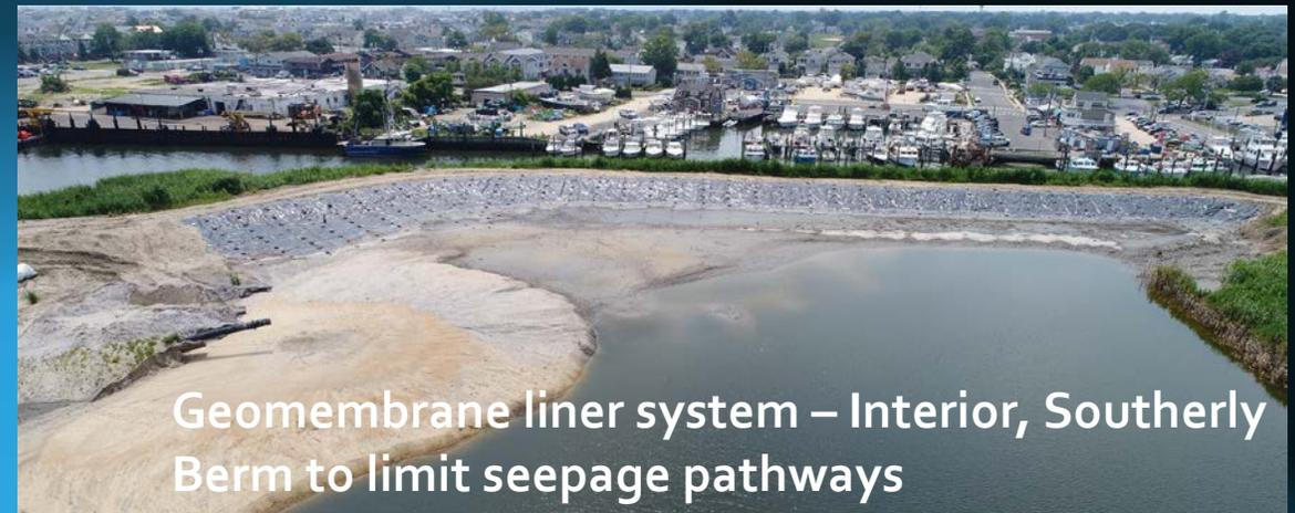
Geomembrane liner system – Interior, Southerly Berm to limit seepage pathways
