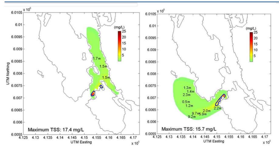
Model-derived SSC (mg/L above background, maximum value in the water column) at ebb flow (left panel, 21:00 January 12) and at flood flow (right panel, 21:00 January 12).
