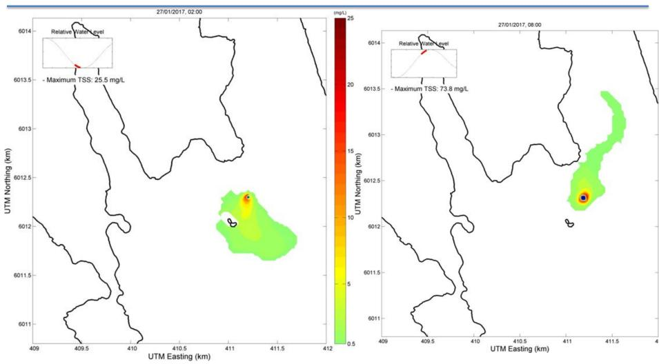
Model derived maximum SSC values in the water column on January 27 following an ebb tide (left panel) and following a flood tide (right panel)
