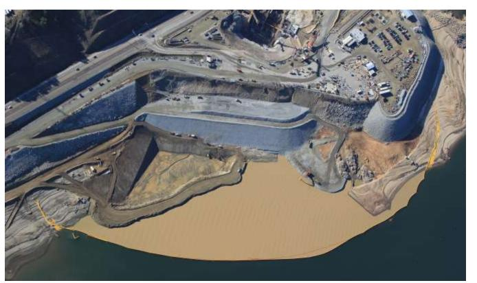
work zones to complete a new spillway offering 4,800' Phase 1 and 2,500' Phase 2 of Type 3 turbidity curtains
