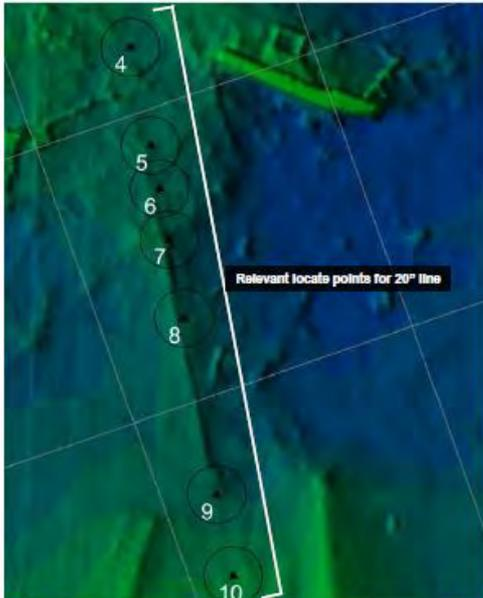
Locate data points overlaid onto a multibeam sonar surface image shows correlating evidence of line exposure.
