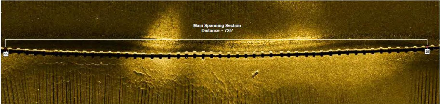
Locate data points portrayed in congruence with side scan sonar imagery confirms a spanning section of pipeline with attached river weights still resting on the lake bed.
