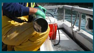
Removing sample from vibrocore
