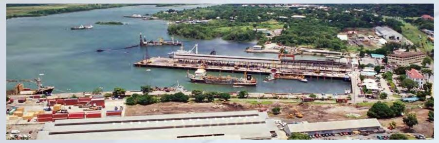
The phases 1 and 2 considered the call of post-panamax vessels with 14.00 m draft, 315 m length and 36 m wide. As a result of the simulations it was decided to dredge the berth pocket at -16.00 m.
