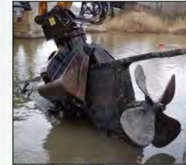
Propeller guard and hull skeg, from one of the tug vessels, stern view.
